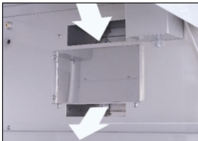
The door is closed, and the system continuously circulates the chamber atmosphere through the wafer system.
