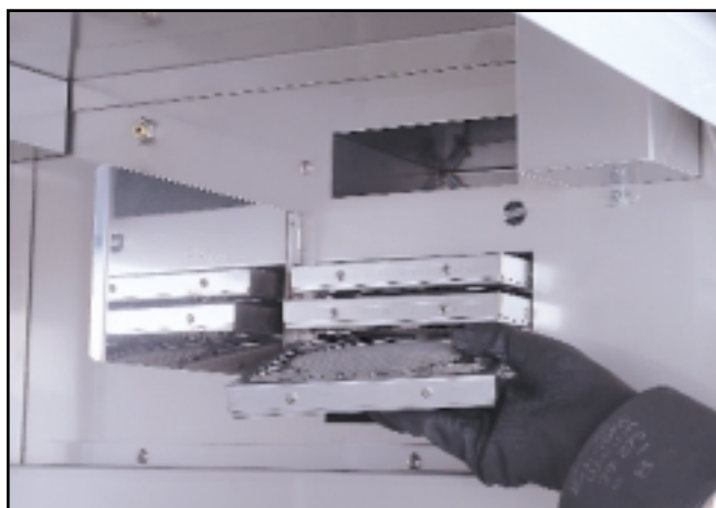
All three wafers are inserted into the airflow system.
