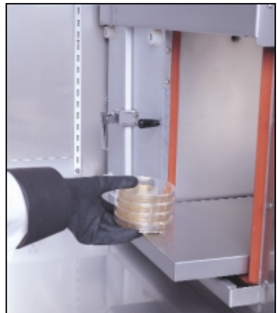
Inner door may be opened and materials moved into the work chamber when the status light on the control panel indicates an anaerobic atmosphere.
