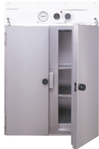
Built-in incubator for incubation capabilities within the anaerobic environment
